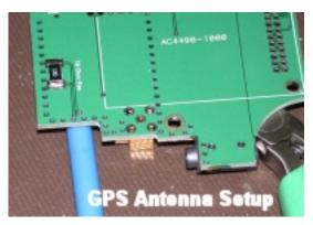
3. While holding the jack in place, invert the PCB (i.e., bottom-side up) and place the PCB, with jack still inserted, on a heat-safe surface (Note: jack will get quite hot during soldering). Use shims to position the height of the PCB above the surface so that the contacts of the jack protrude slightly and evenly above the bottom-side of the PCB.
