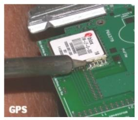
the remaining pads on the PCB. Repeat this tacking procedure on a contact in the opposite corner of the GPS.
