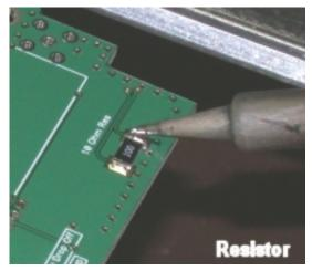
a length of solder (held in the off-hand) to supply ample solder to the joint. Repeat on the tack joint of the opposite end. This is a small part so, be careful not to allow the iron tip to linger on the part.
