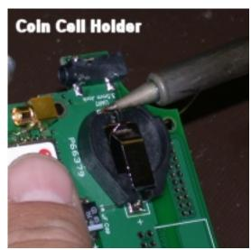
3. Using a clean iron tip, apply heat to one of the contacts until solder becomes molten and wicks under and around the contact when touched to the heated contact. This may take a while because the contacts on this part are large thus forming substantial heat sinks. This part is not particularly heat sensitive but the plastic portions with melt if you hold the iron against them.
