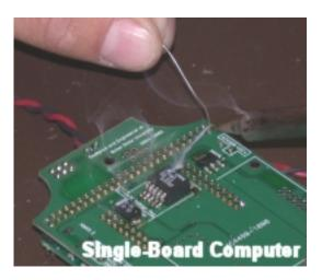
5. Using a loaded iron tip, tack one of the contacts located at one end of the 50-pin header to its plated hole. Move to a contact on the opposite side of the computer from this first contact and tack down this second contact.
