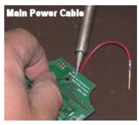
push the wire back down into the hole so that the insulation is in contact with the top rim of the hole.
