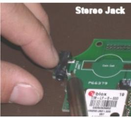
4. Use ample solder to re-solder the tack joint involving the first contact. Inspect the quality of all 3 joints and correct, if necessary.
