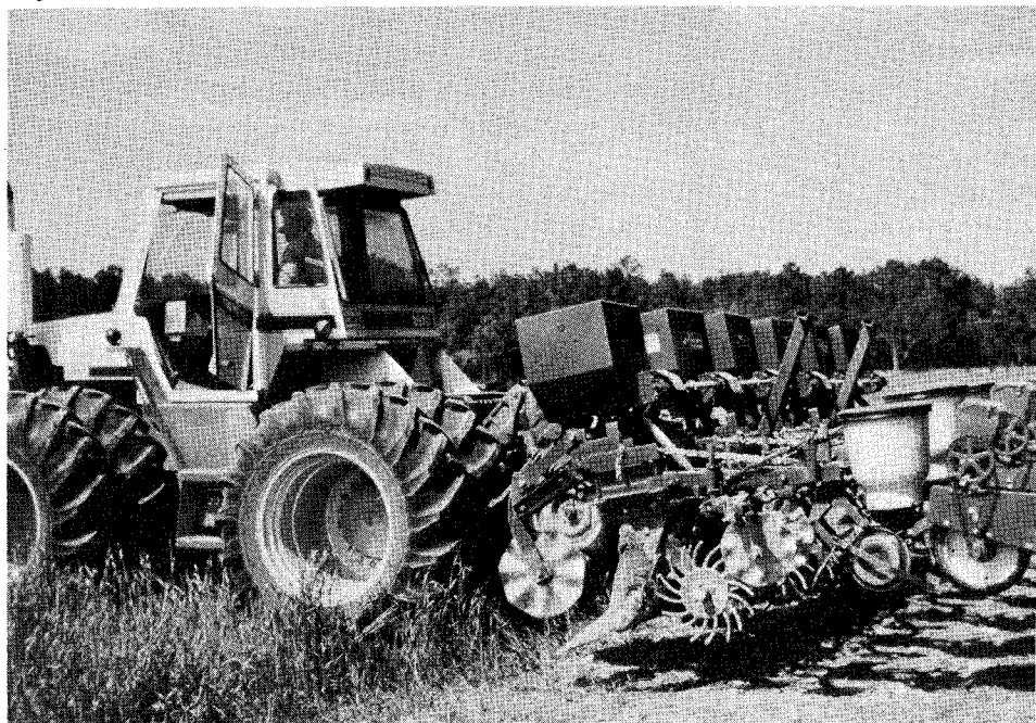
Fig. 1. Six-row conservation tillage planter equipped with dry fertilizer distributors, insecticide hoppers, and a rear-mounted herbicide spray system (not visible).
