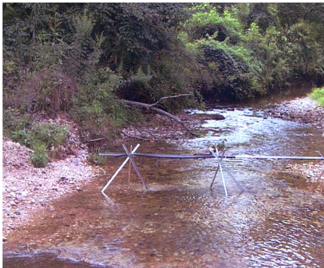
Figure 2. Photograph of the injection apparatus in Cloud Creek during an injection pilot run.
