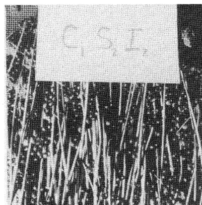
FIG. 1 Trays of Clods after Treatment and drying. Variables shown are: straw cover, 50 (C 1 ) and 90 (C 2 ) percent; hail diameter, 1.64 cm (S 2 ); and hail energy, 0.53 (I 1 ) and 2.10 (I 2 ) cm-newtons cm -2 .
