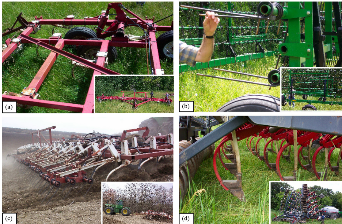
Fig. 2. Photos of the four tillage implements: (a) deep-tiller; (b) spring-tooth-harrow; (c) light-cultivator; (d) air-seeder.
