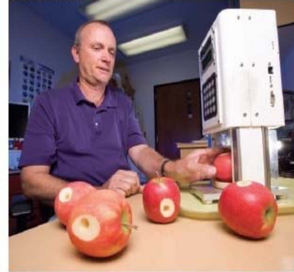
Technician David Buchanan uses a recording penetrometer to measure apple firmness, a key component of apple fruit quality.
