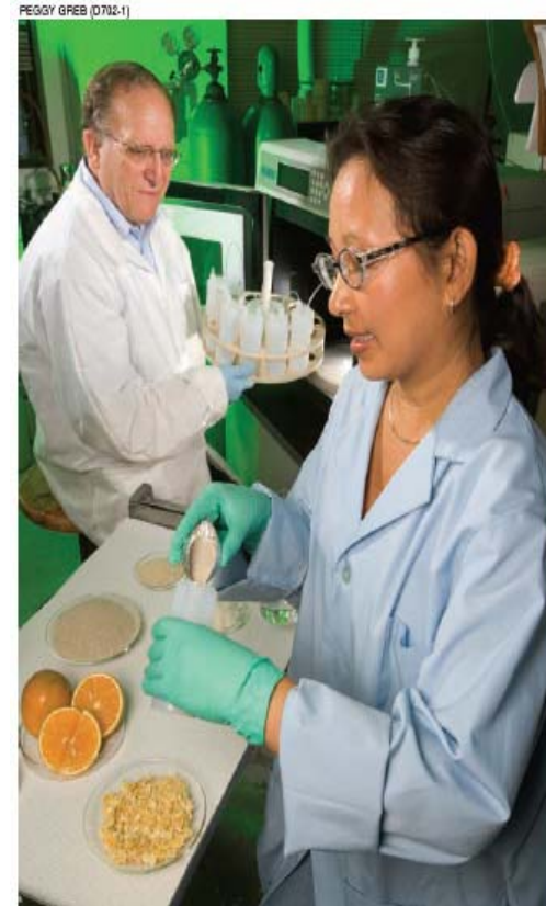
Chemists Marshall L. Fishman (left) and Hoa K. Chau prepare orange peels for flash extraction of pectin using microwave heating under pressure.
