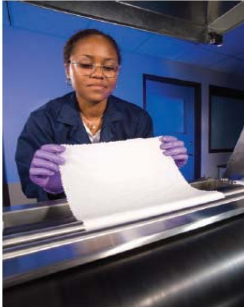
Chemist Nicolette Prevost treats cotton fabrics with a chitosan formulation, which is designed to confer blood-clotting and antibacterial properties on wound dressings and specialty garments.
