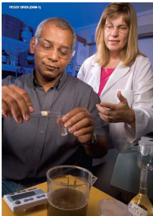
Chemist Gillian Eggleston (right) demonstrates the simple, rapid enzymatic mannitol test to Hedgardo M. Centella, a factory laboratory technician at Alma Sugarcane Factory, Lakeland, Louisiana. A spectrophotometer is required for the test.
