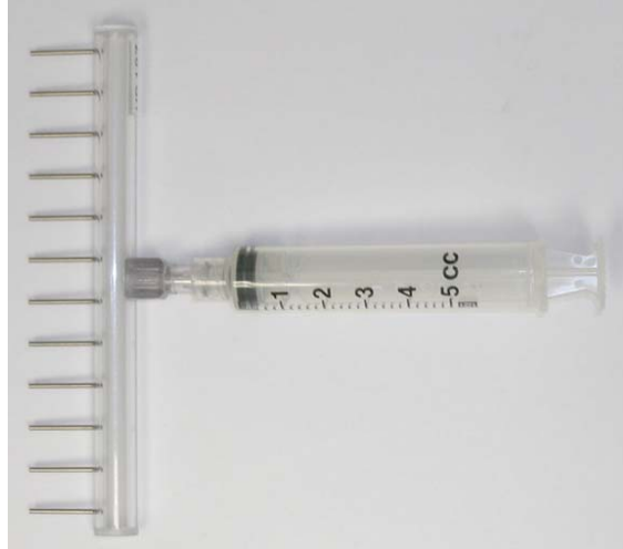
Figure 1. Recently my laboratory has been using a 12-channel manifold attached to a syringe with the plunger all the way down to prevent capillary action from drawing any sample out of the well to mix the dye with the protein sample. This reduces the mixing time and does not cause bubbles to form as does occur when mixing with a multi-channel pipette. Caution must be used to make sure the bottom of the well is not scratched. To prevent scratching, stir in a circular motion with the manifold sitting just above the bottom to mix horizontally and move straight up and down touching the bottom to mix vertically.
