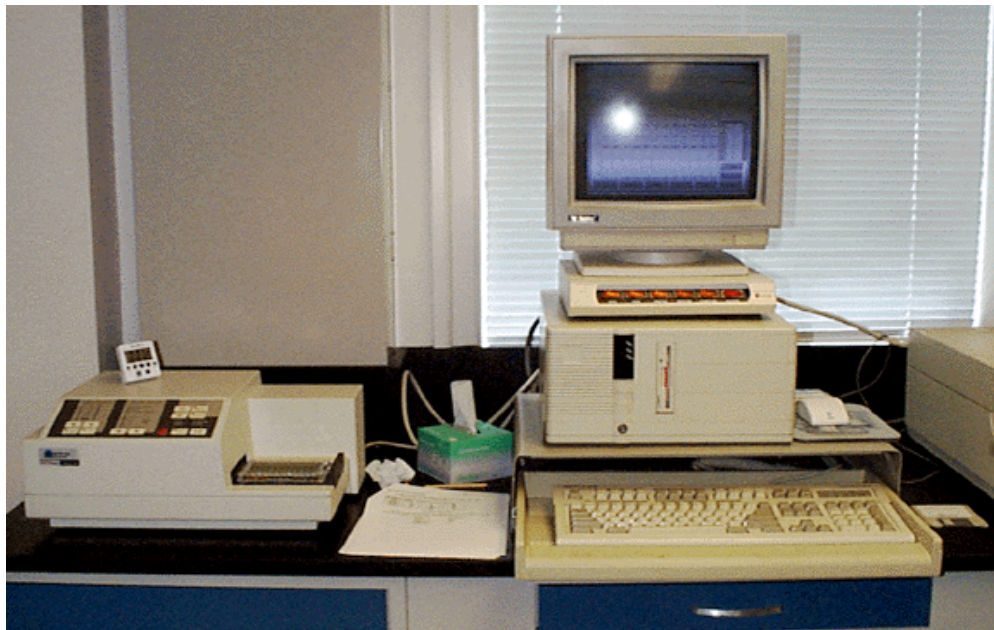
Figure 2. Typical computer and plate reader set-up for the Bradford total protein and ELISA immunoreactive protein assays. Software that either comes with the plate reader or may be purchased separately may be used to assist in the analysis of the data. We use Softmax® software. If software is not available or a computer interface is not available, data may be collected directly from the plate reader and inputted into a spreadsheet program, like Excel, for analysis.
