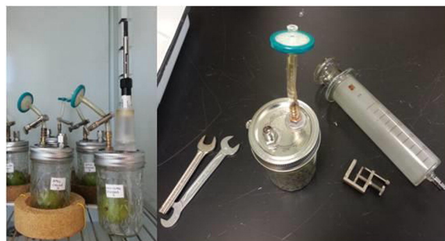
Fig. 1. Volatile collection system (semi-closed system) used to collect ex-situ walnut volatiles by HS-SPME and the venting set up used for headspace exchange after each HS analysis.
