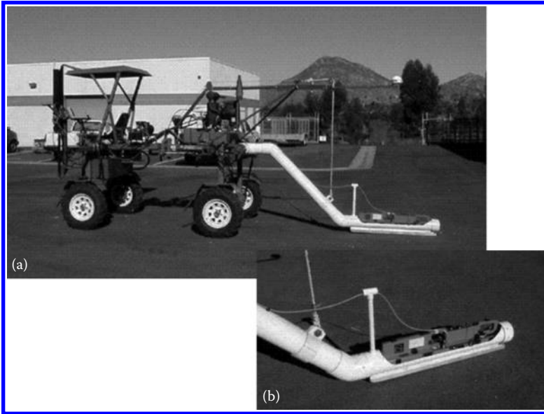
FIGURE 8.6 Mobile GPS-based EMI equipment showing (a) a side view of the entire rig and (b) a close-up of the sled holding the EMI unit.
