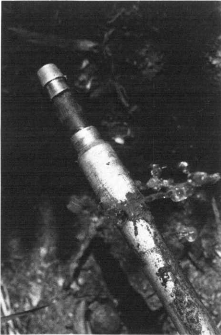
Fig. 3. Barbed fitting at the end of the pipe used for jetting a hole from the trunk of each tree to the trench containing the corrugated pipe. The delivery hose is slipped over this fitting and is thereby drawn into the hole when the jetting pipe is retracted.
