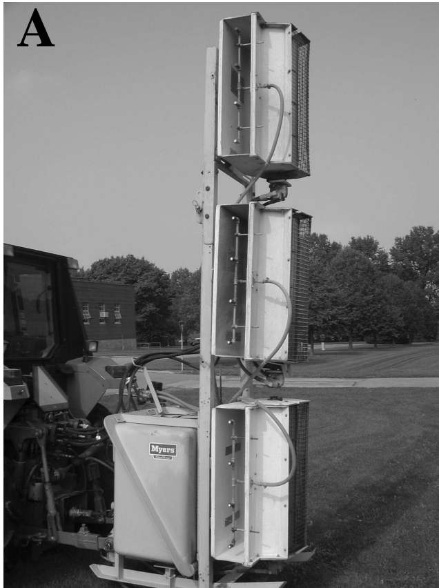
Fig. 1. Experimental, three fan, cross-flow (CF) sprayer used in nursery trials: A) CF sprayer with all fans oriented to produce horizontal air-flow and B) single CF fan assembly with five nozzles positioned at the fan outlet.
