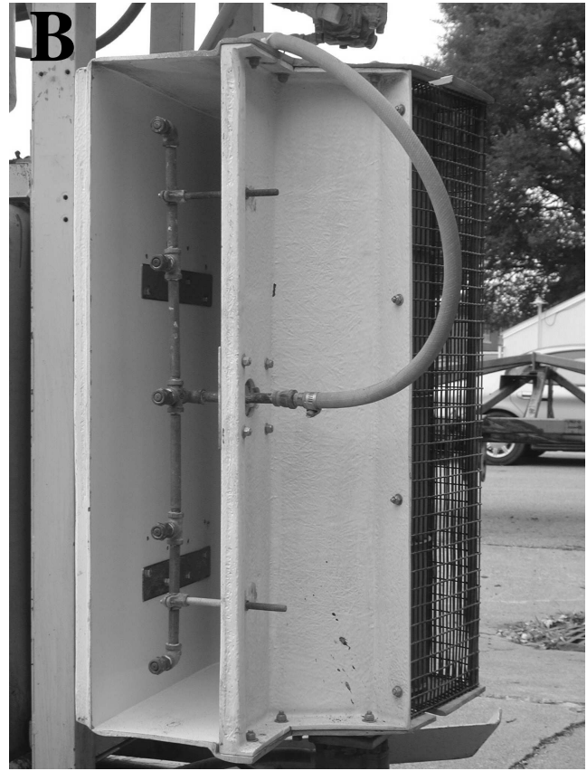
Fig. 1. Experimental, three fan, cross-flow (CF) sprayer used in nursery trials: A) CF sprayer with all fans oriented to produce horizontal air-flow and B) single CF fan assembly with five nozzles positioned at the fan outlet.
