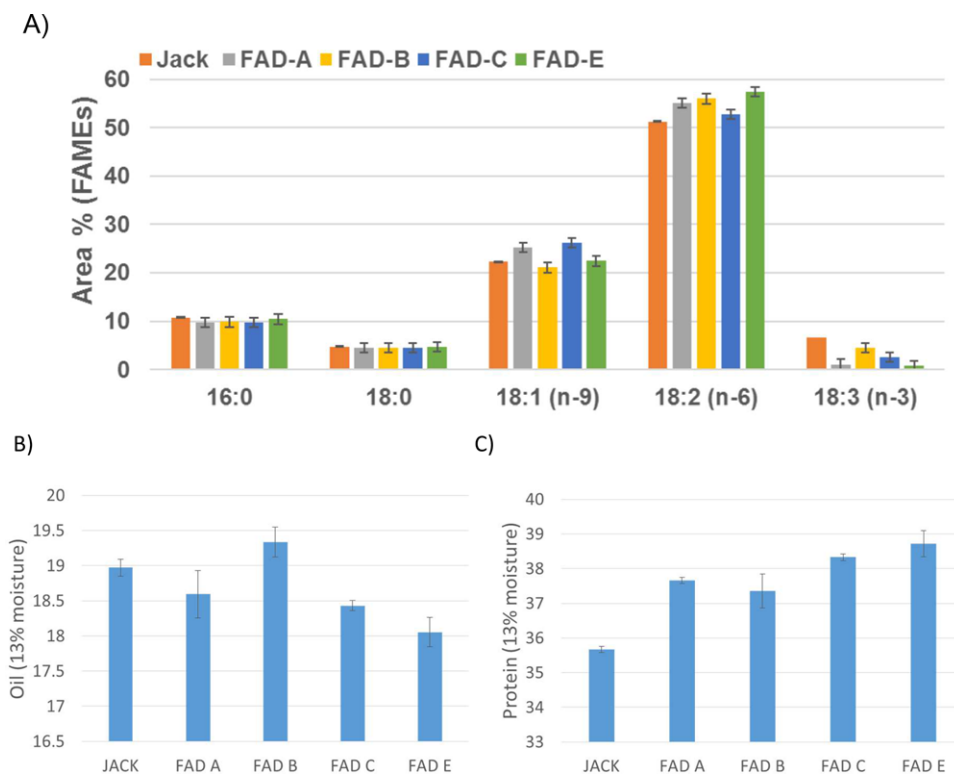
Figure 1. A) Fatty acid methyl esters analysis by gas chromatography–flame ionization detector of the transesterified oil extracted from five sets of soybean samples; B) total oil content of the five soybean samples and; C) total protein content of the five soybean samples determined by NIR.
