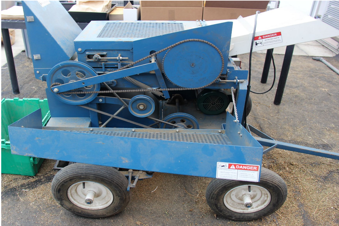
Belt threshing rig at PGRU
