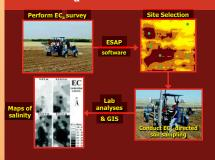
Typical EMI EC<sub>a</sub> Survey and Site Selection to Quantify Field-Average Salinity:
