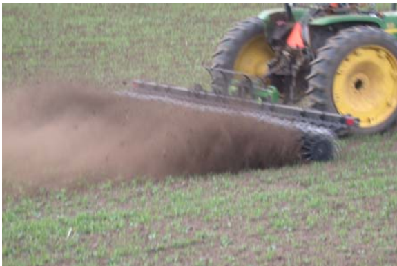
Rotary hoeing an emerged cover crop at 8-10 mph
