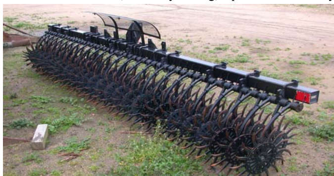
15' wide Yetter Rotary Hoe. Cost \approx $2,500
