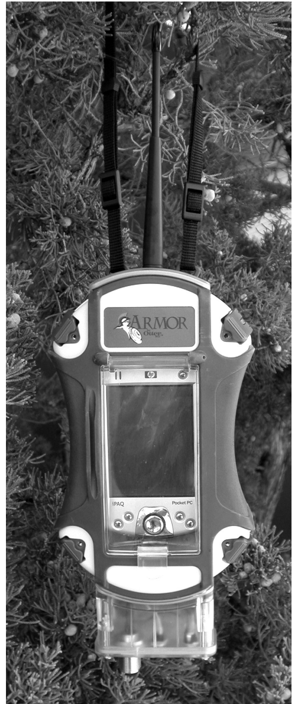
Figure 2. The Clark global positioning system Animal Tracking System hand-held base station including personal digital assistant, spread-spectrum radio transceiver, and waterproof case.
