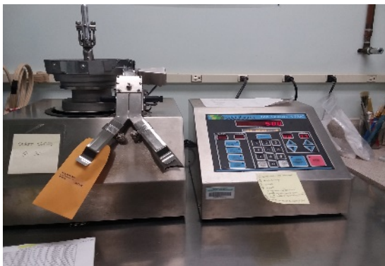
Figure 4: Seedburo 801 Count-A-Pak set up for seed count.
