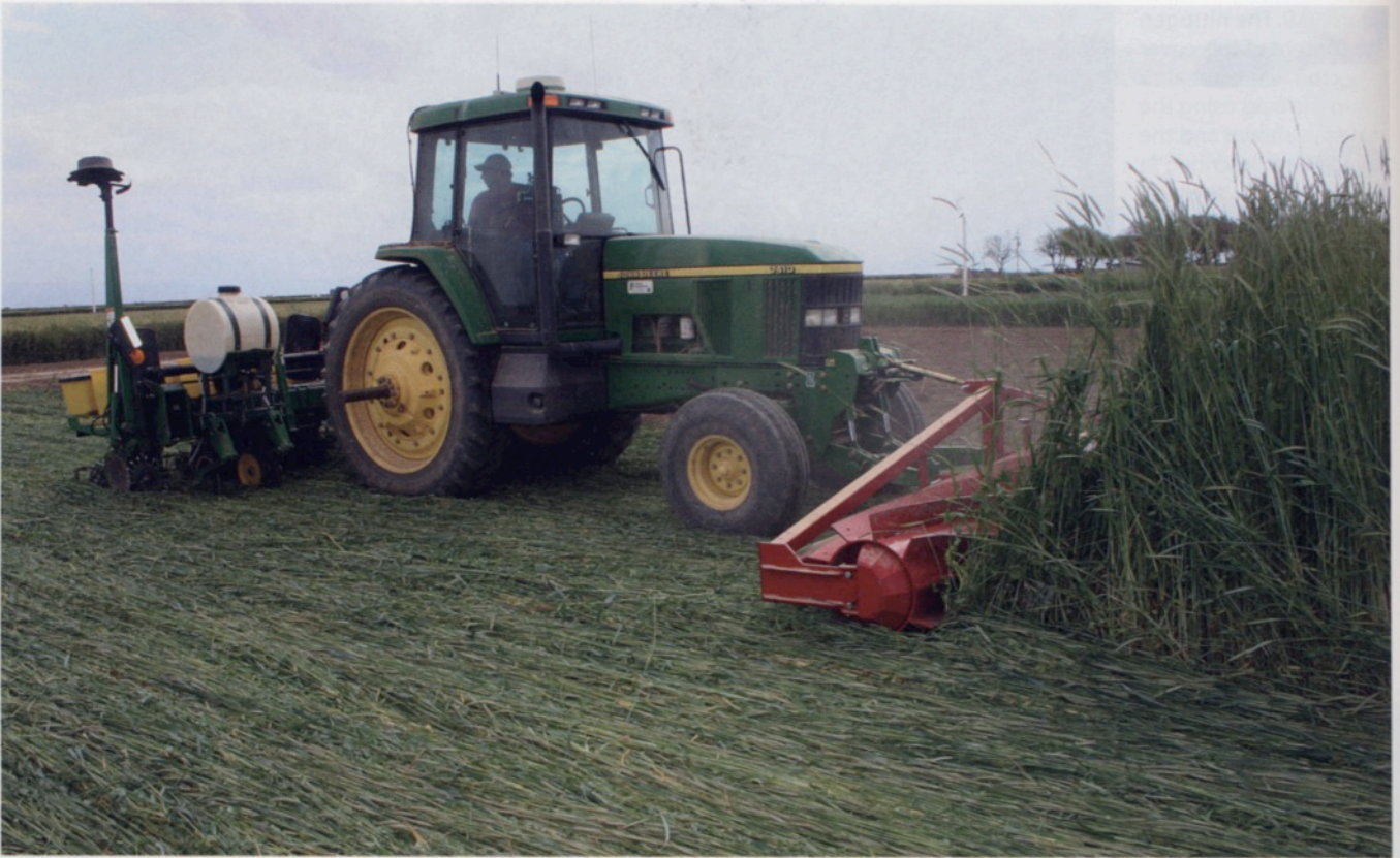
Figure 10.12. Front-mounted roller-crimper flattens rye cover crop while rear-mounted seeder plants cotton. J. MITCHELL.
