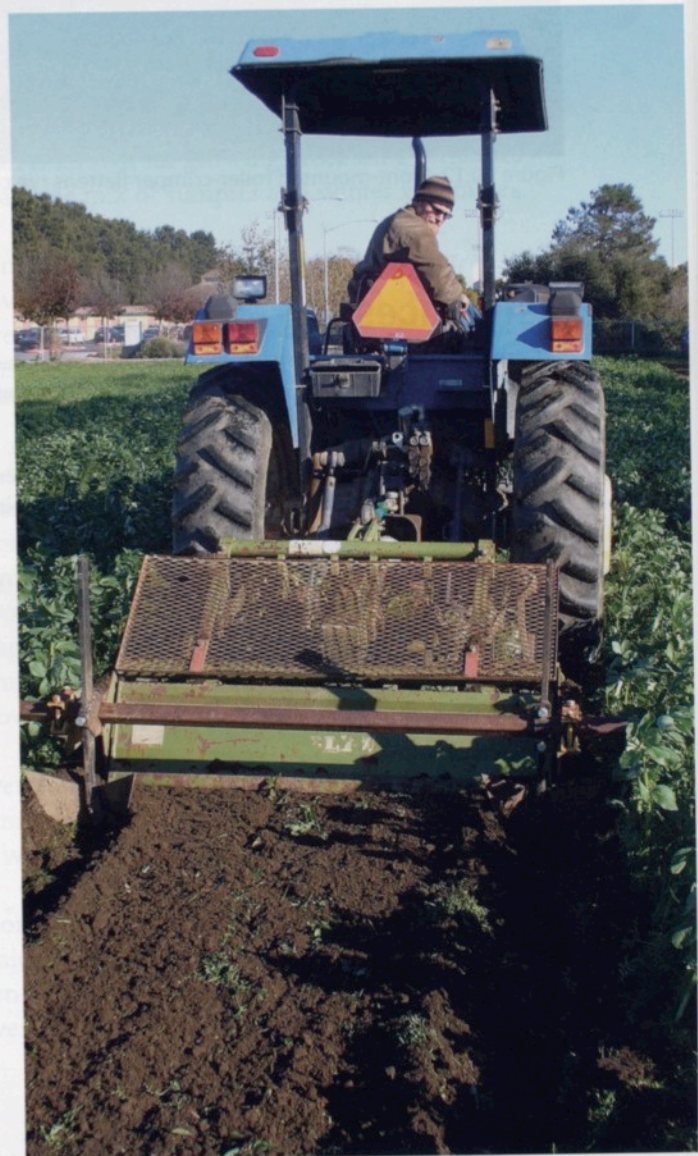
Figure 10.11. A spader incorporates standing cover crop of mixed legumes in one pass. M. VAN HORN
