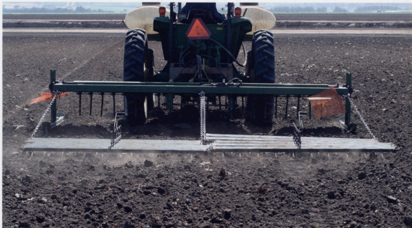
Fig. 10.3. Broadcasting mustard seed on the soil surface from a small, hydraulically driven seed hopper and shallowly incorporating it with a spike-tooth harrow. R. Smith
