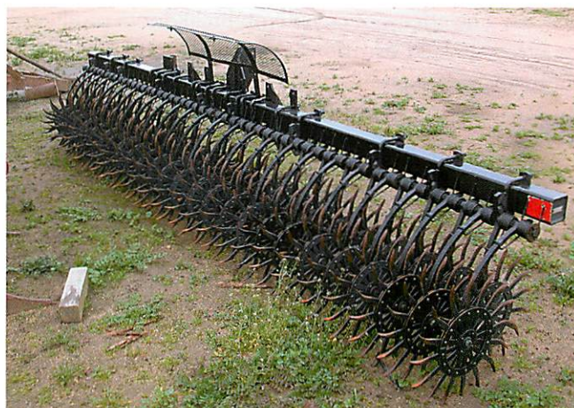
Figure 6.3. Rotary hoe implement used for blind cultivation.
