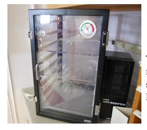
Then seeds are put into coin envelopes for final drying to 5% without added heat in a silica gel desiccator, e.g., SanpiaTech® DryKeeper. After drying, any chaff or flat seeds present is removed with, e.g., an Oregon Seed
