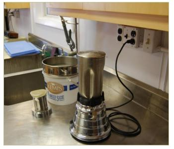
The pulp and seeds are poured from the blender into a round sieve (~2mm holes) over a plastic pail. Then tap water is sprayed from a standard food service sink nozzle to separate seeds from the pulp and force the seeds through. Remaining unwanted tissue and slime that passes the seive can be removed by repeated rinsing and decanting (seeds settle to the bottom).
