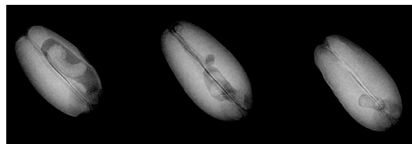
Figure 2. X-ray image of internally infested wheat showing examples of large, medium, and small larvae.
