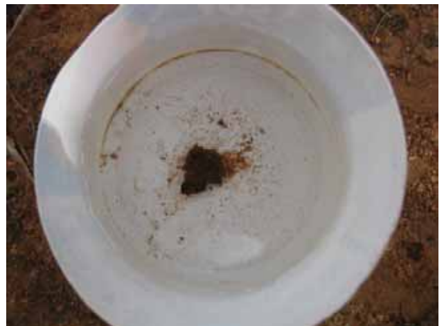
Soil sample that has remained stable, even after swirling it
