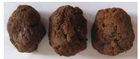
Examples of soil samples collected from three different depths: 0-10 cm (left), 10-30 cm (middle), and 30-50 cm (right). The darker surface soil indicates that there is more organic material in the soil at the surface.
