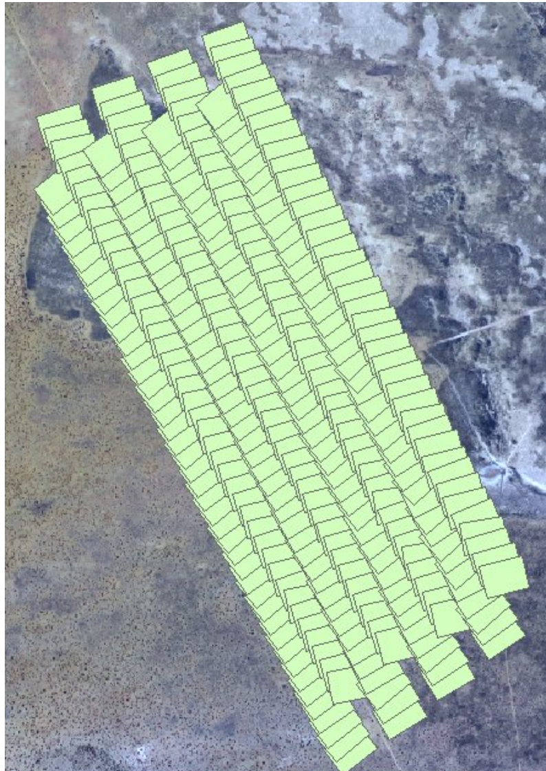
Fig. 6. Footprints of BAT UAV imagery overlaid on QuickBird image.
