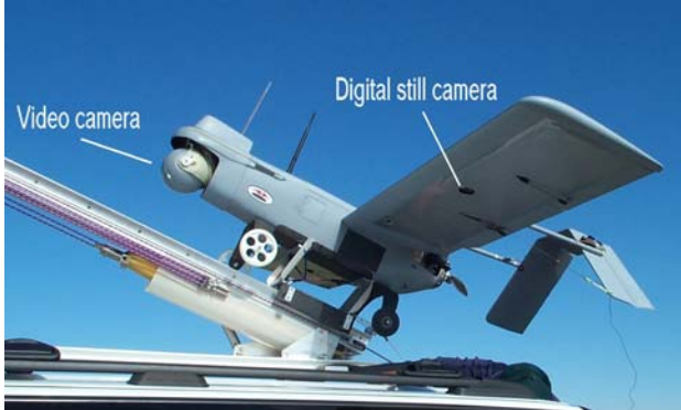
Figure 1. BAT 3 UAV on catapult on roof of launch vehicle. The video camera is located at the front; the digital still camera used in this study is located in the left wing.
