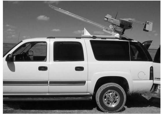
Fig. 1. BAT 3 UAV on catapult launcher ready for takeoff.
