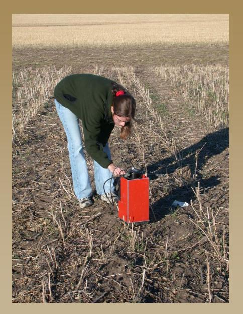
We used a neutron moisture meter to measure soil water contents. The active part of this instrument is lowered into a tube in the soil to take readings at approximately weekly intervals.
