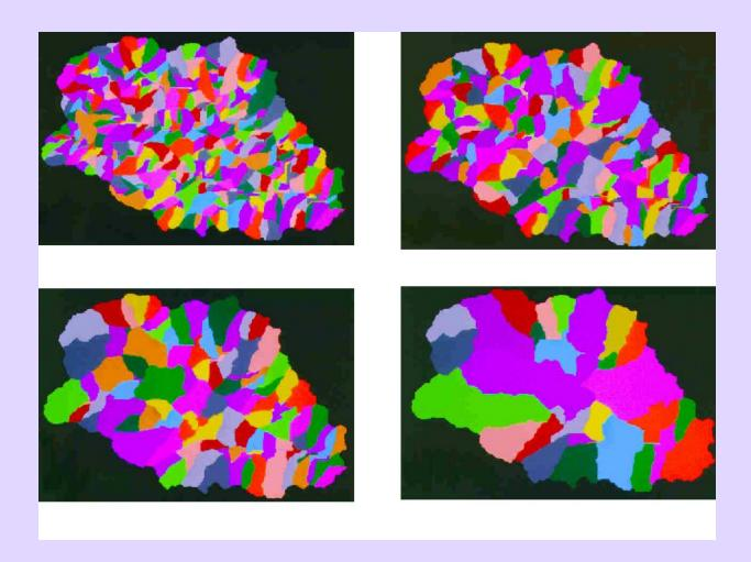
This image illustrates the difference in generated subcatchment resolution as a result of different values of the Critical Source Area (CSA). The CSA parameter represents the threshold drainage area below which as channel is assumed to form. Small CSA values produce small subcatchment areas, and large values produce large subcatchment areas. The image was created from information produced by TOPAZ.
