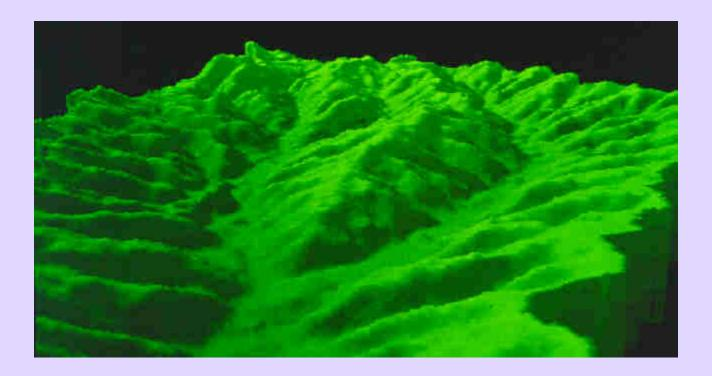
This is a 3 dimensional representation of the Digital Elevation Model of a watershed. The image was created from information produced by TOPAZ.
