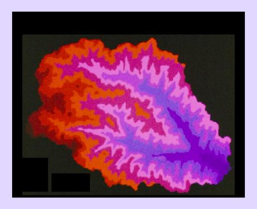
This image displays areas of elevations that fall within a user-specified range of elevation values. Blue colors represent lower and red colors higher elevations. The user can select any number of elevation classes to produce images that meet the needs of specific applications. The image is based on information produced by TOPAZ.
