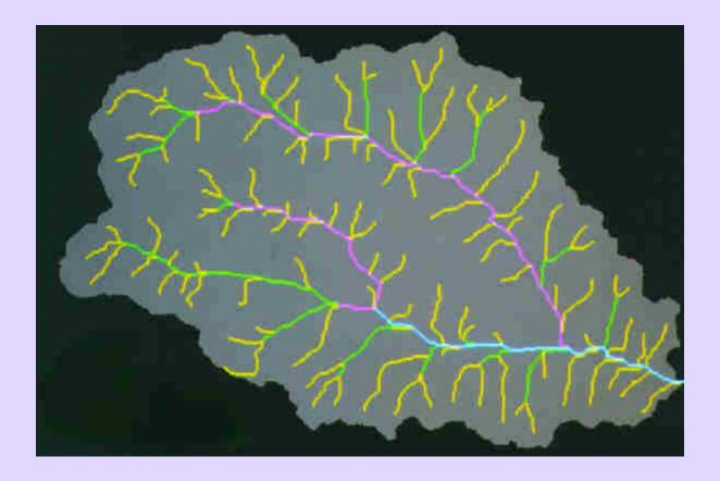
This is a display of the generated channel network within a watershed area. The different colors in the channel network represent the different Strahler orders of each channel link. The image was created from information produced by TOPAZ.
