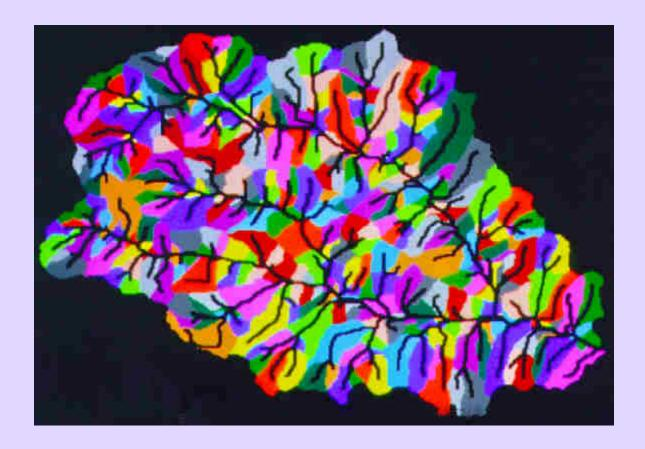
This image displays the enhanced network and catchment areas. The channel network has been enhanced (widened) for better visualization. The source, right and left subcatchment areas have been aggregated into one catchment area for each channel link. The image was created from information produced by TOPAZ.
