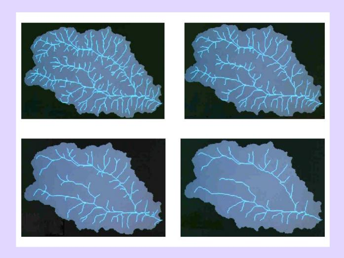
This image illustrates the difference in the drainage density of the generated network by changing the value of the Critical Source Area (CSA) from a smaller to a larger area value. The CSA parameter represents the threshold drainage area below which as channel is assumed to form. The image was created from information produced by TOPAZ.
