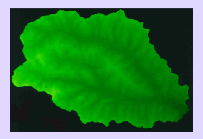
This image displays elevations of a Digital Elevation Model (DEM) within a given watershed boundaries. Dark green colors represent lower elevations and light green colors higher elevations. The image is generated from a standard USGS 30 meter DEM. DEMs are a basic input to TOPAZ. The image was created from information produced by TOPAZ.
