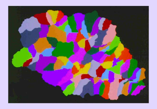
This image displays subcatchment areas. Each subcatchment area drains into a channel link. The image was created from information produced by TOPAZ.
