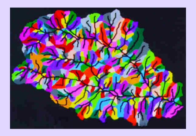
This is a display of the enhanced generated channel network within a watershed area overlaying aggregated subcatchment area. The network has been enhanced for display by a general widening applied to the entire network. The subcatcment areas have been aggregated from source, left and right areas into a single subcatchment area. The image was created from information produced by TOPAZ.
