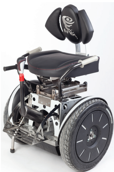
FIGURE 3-7 Segway modified to serve as a wheelchair.
