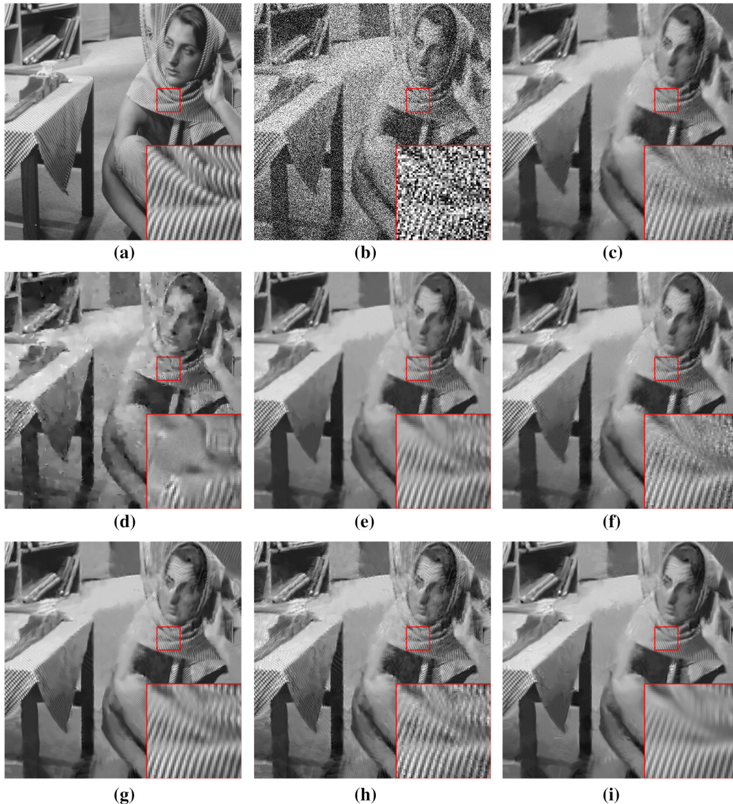
Fig. 9 Denoising results on image “Barbara” by different methods ( \sigma = 7 ): (a) ground truth (PSNR/SSIM), (b) noisy image (10.63/0.1118) (c) BM3D (25.37/0.7112), (d) EPPL (29.98/0.6887), (e) FRIST (23.57/0.7302), (f) WNNM (23.62/0.7421), (g) STROLLR (23.46/0.7287), (h) PGPD (23.60/0.7397), and (i) EPL-IMSC (23.69/0.7476).
