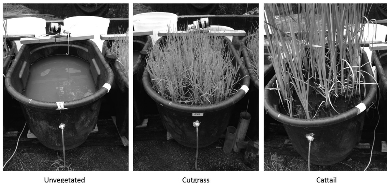
Fig. 1. Experimental mesocosms under different vegetation treatments. From left to right: unvegetated control, cutgrass [ Leersia oryzoides (L.) Sw.], and cattail ( Typha latifolia L.). Each treatment had three total replicate mesocosms.
