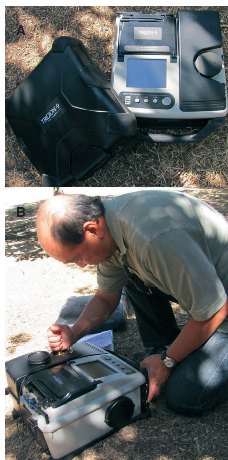
Figure 1. The hand-held portable GC-MS with case (A) and an adsorbed sample being thermally desorbed (B) onto the GC-MS from the needle trap/holder assembly.
