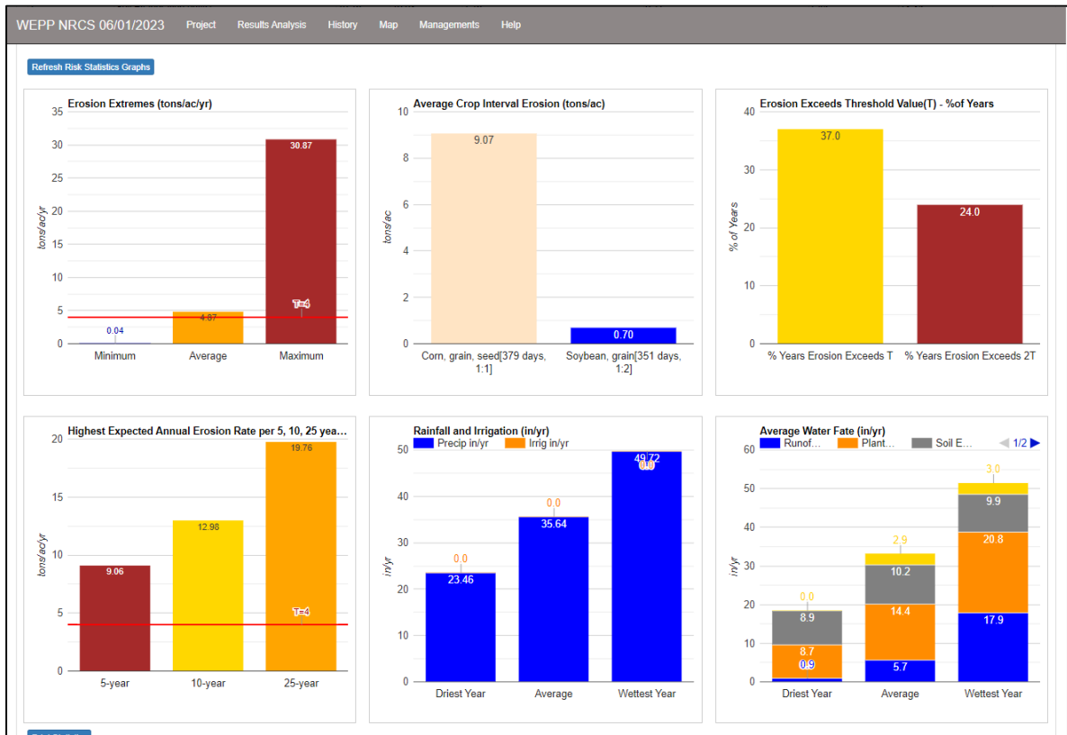
Figure 3. Some of the graphical outputs from web-based interface for NRCS field office soil conservation applications. Results shown here highlight results from 100-yr simulation and recurrence interval values. Notice the much greater soil loss predicted during the corn part of the rotation where substantial tillage occurs (top center figure).
