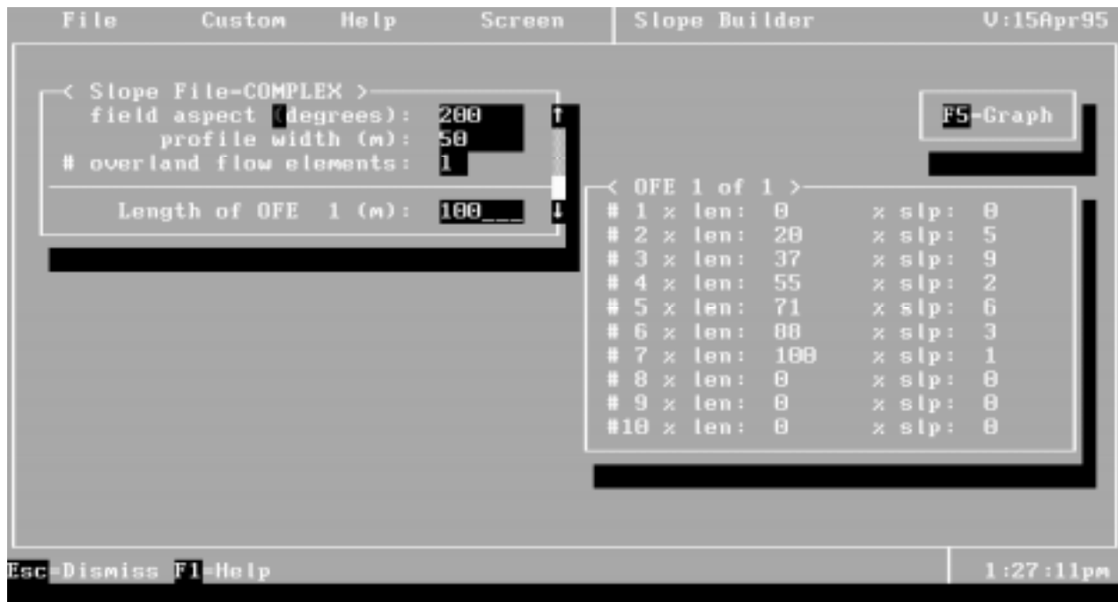
Figure 24. Main screen of slope input file builder with pop-up screen for point slope entry for OFE 1 shown in lower right hand corner.
