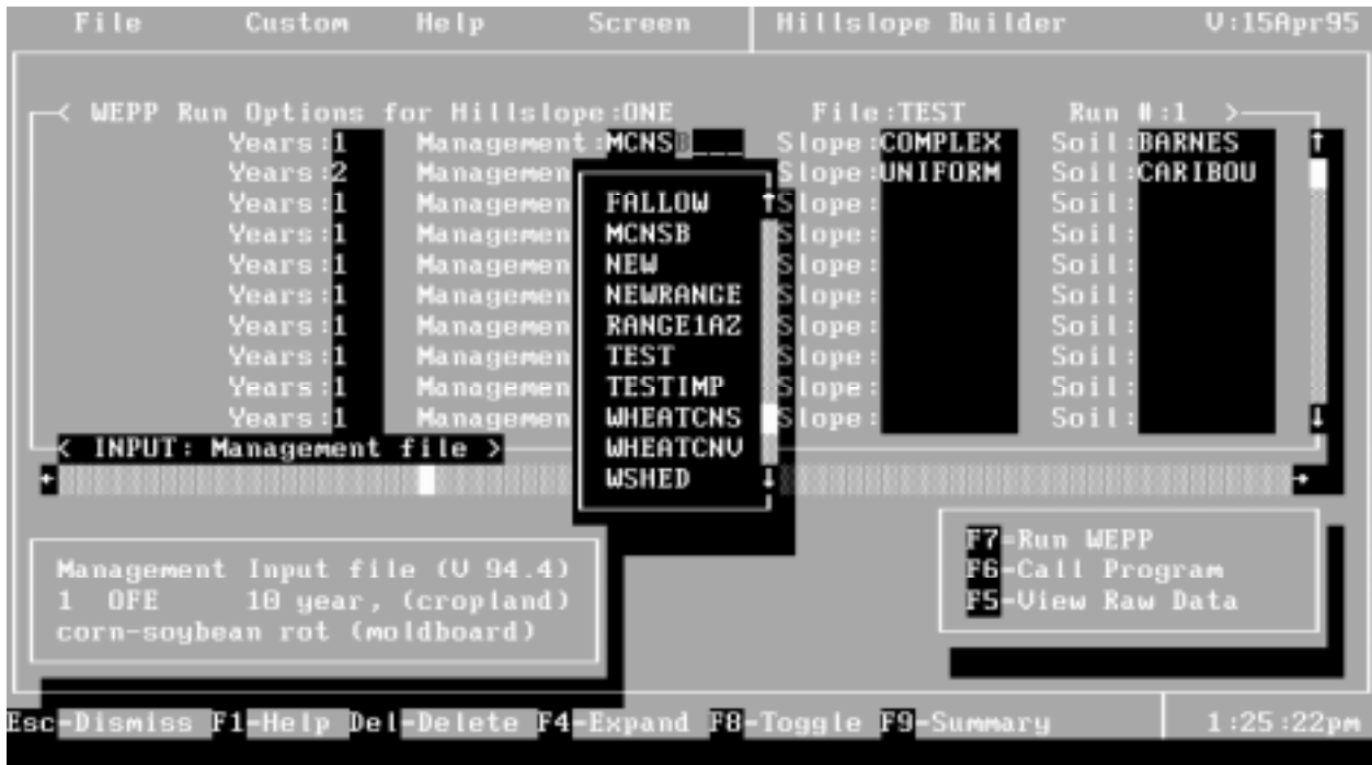
Figure 21. Portion of the WEPP Hillslope Interface run definition table with WEPP input data fields and expanded plant/management file selection list.
