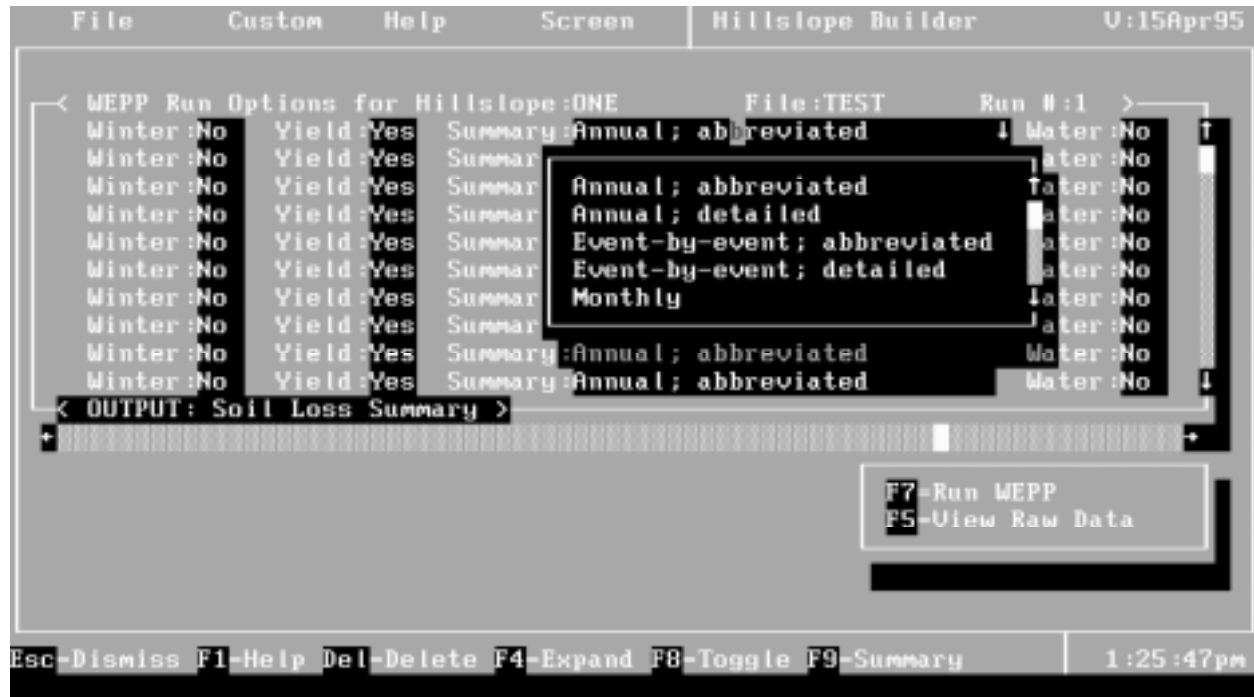
Figure 22. Portion of the WEPP Hillslope Interface run definition table showing the WEPP model output option selection and expanded list for the runoff/erosion summary output type.
