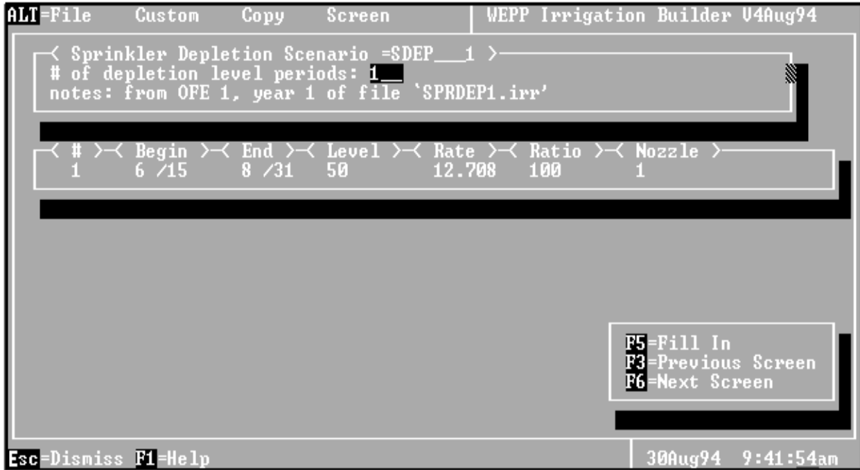
Figure 33. Irrigation file subscreen illustrating the table of values required for Depletion-level Sprinkler irrigation.
