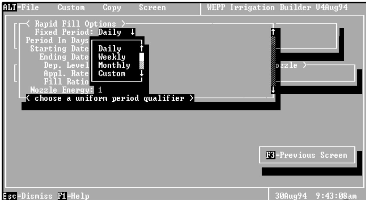
Figure 34. Irrigation file subscreen illustrating the rapid fill feature under Depletion-level Sprinkler irrigation
