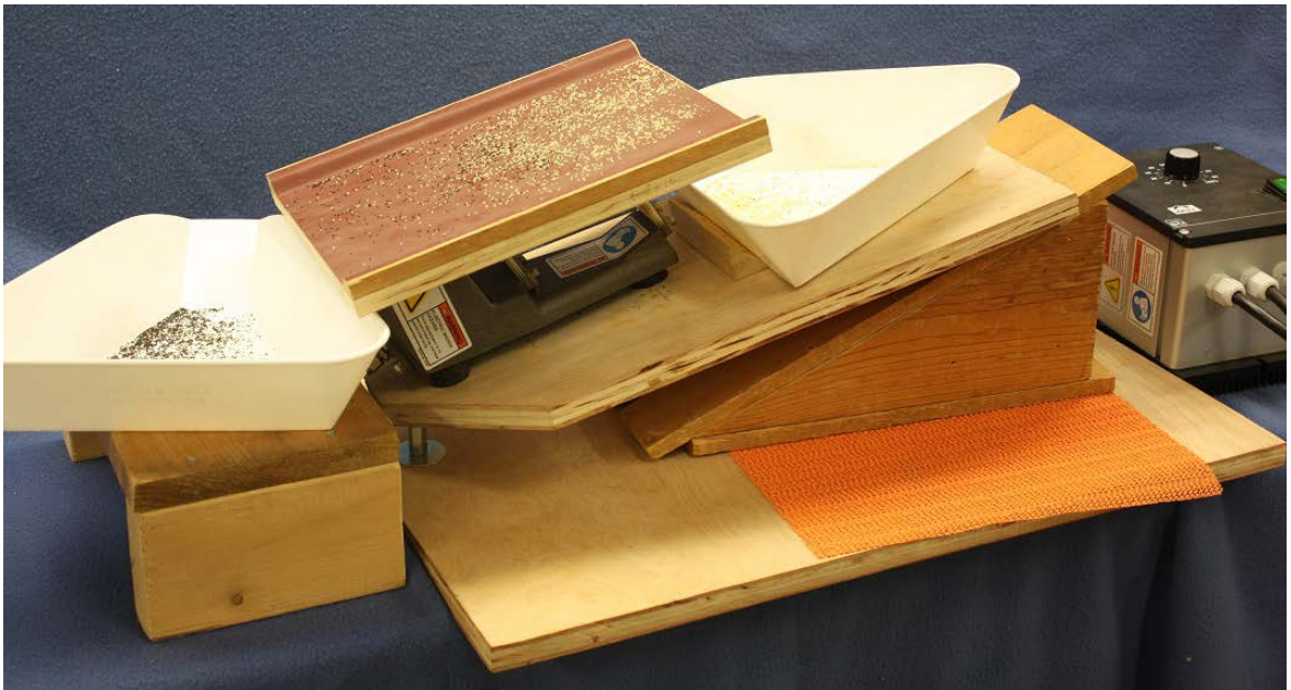
A vibratory deck seed cleaner with newly constructed wooden and plywood gear built by David Brenner.
