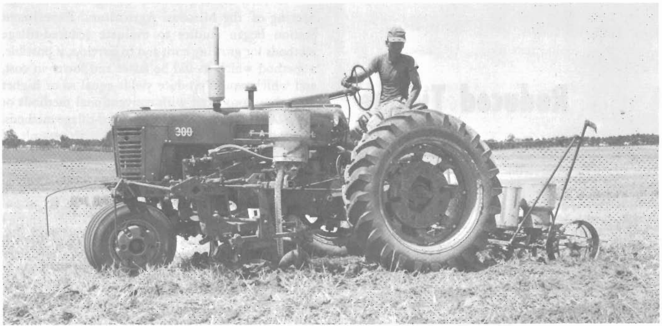
Fig. 1 The once-over strip tilling and planting equipment used in the first experiments on reduced tillage. The strip tiller equipment, mounted on the tractor cultivator frame, consists of wide sweeps to clear trash from the row areas,
