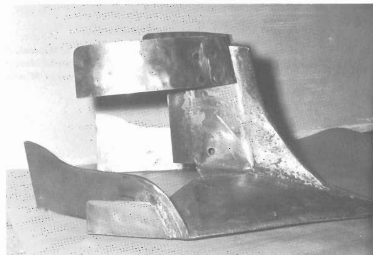
Fig. 2 The basic strip plow unit which was developed from these studies. The top wings force the surface soil and trash outward, and the lower wings move moist, trash-free soil in the bottom of the furrow slice toward the center of the strip.
