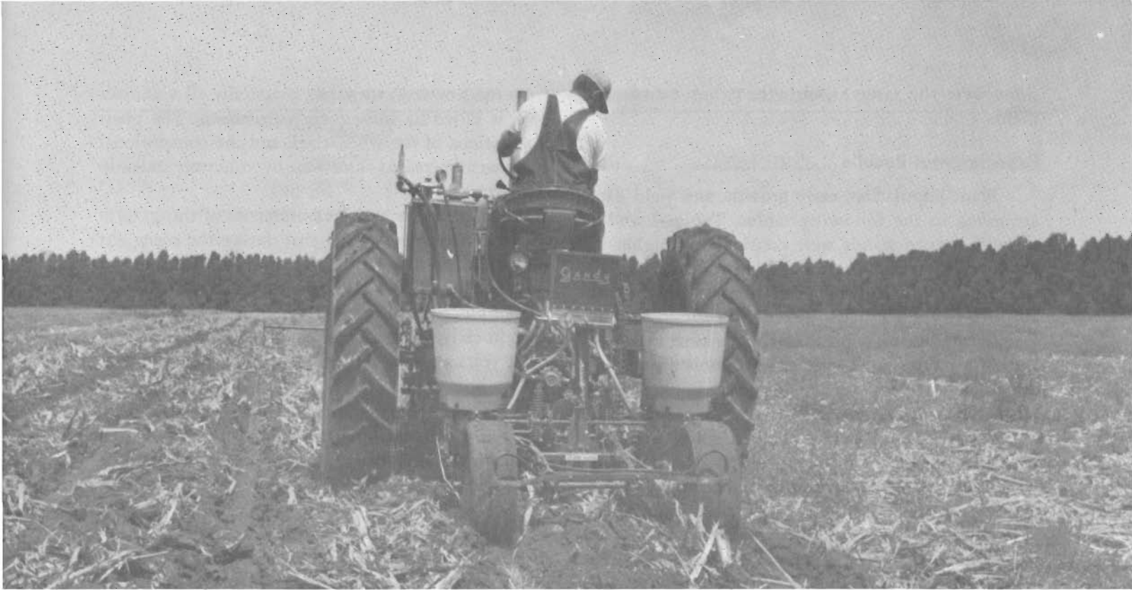
Fig. 5 The strip plow and planter at work. Stalks from the previous crop were shredded, but no other work was done ahead of the strip plow. The strip plow units are mid-mounted ahead of the tractor rear axle, and a tractor planter is rear mounted and equipped with attachments to apply fertilizer, soil insecticide, and a herbicide.
