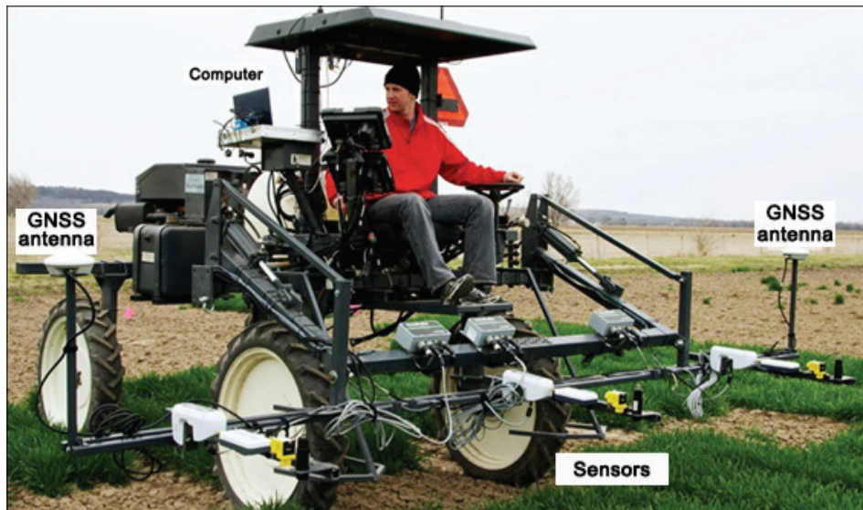
Figure 10. Field-based HTPP platform on a MudMaster sprayer. Three rows of sensor sets are mounted on a hydraulically positioned bar. Two GNSS antennas are located at each bar end.
