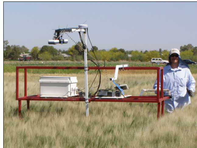
Figure 18. Field-based HTPP platform on a low-cost cart.
