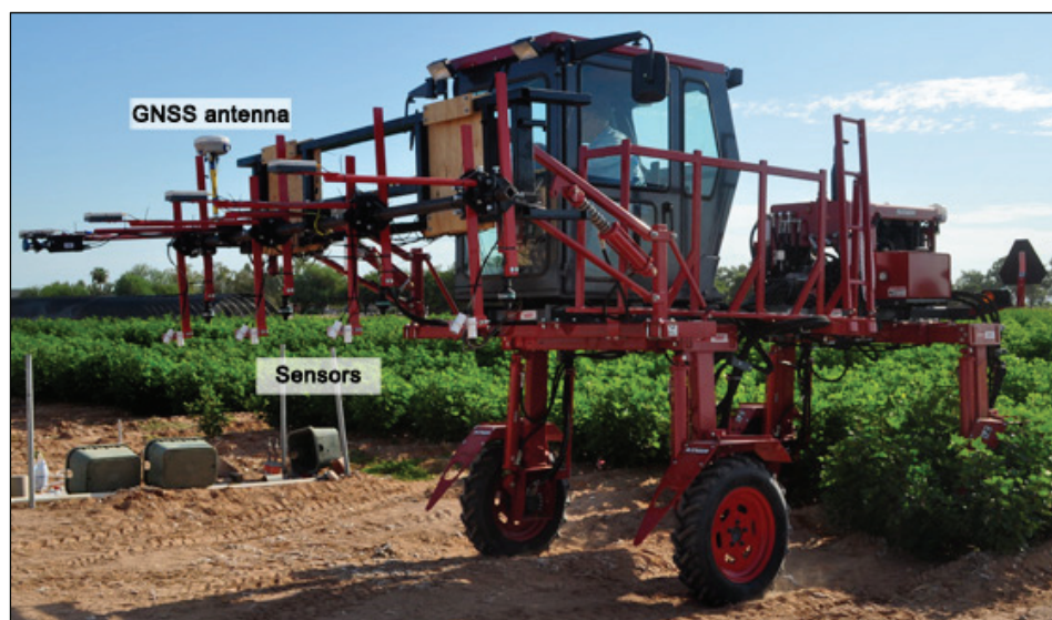
Figure 5. Field-based HTPP platform on a Lee Avenger tractor. Four rows of sensor sets are mounted on a hydraulically positioned bar. The GNSS antenna is located at the bar midline.
