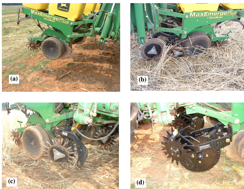
Figure 2. Row cleaners: (a) basic planting unit with no row cleaner, (b) Dawn, (c) Dawn/no couler, and (d) Yetter.
