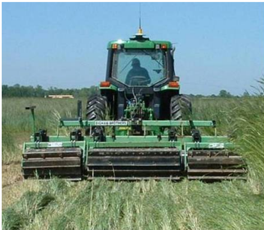
Figure 1. Three-section roller with straight crimping bars 4.1 m wide.
