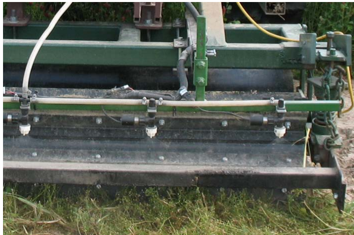
Figure 2. High speed solenoid valves to control nozzle discharge (flat pattern) of herbicides.
