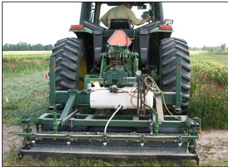
Figure 1. Two-stage roller/crimper with mounted 53 L plastic tank and boom with 5 nozzles each controlled by fast acting solenoid valve to discharge herbicides on crimped cover crop residue.
