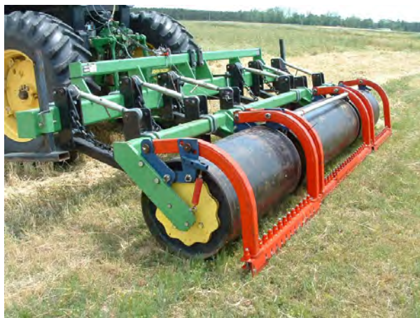
Figure 2. Three-section smooth roller with crimping bar assembly.
