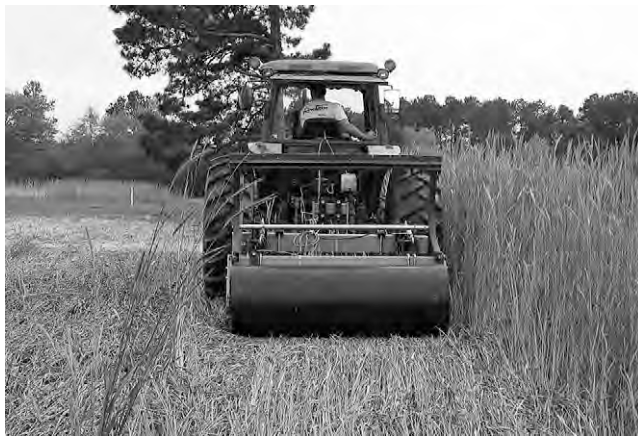
Fig. 5. Smooth roller drum without crimping bars attached.
