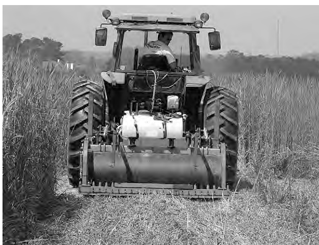
Fig. 3. Smooth roller with crimper. Design developed at the NSDL (U.S. Patent 7,604,067 B1; Kornecki and Raper, 2009).
