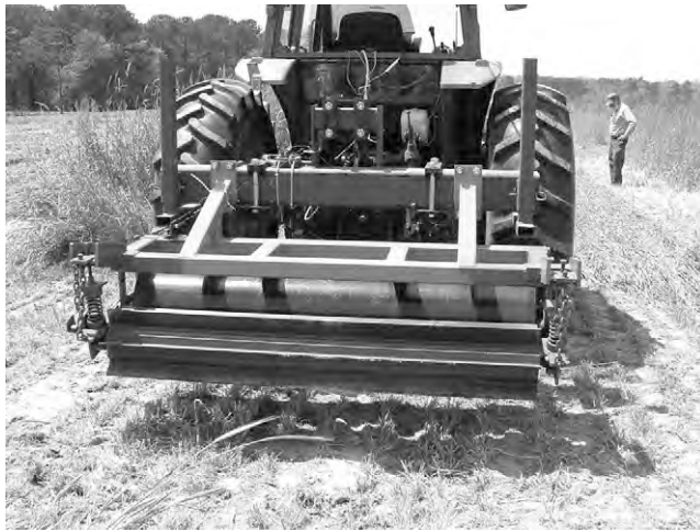
Fig. 4. Two-stage roller comprised of a smooth drum and spring loaded crimping bar drum. Design developed at the National Soil Dynamics Laboratory (U.S. Patent 7,987,917 B1; Kornecki, 2011).
