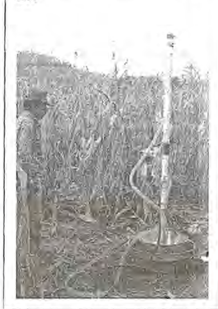
Figure 1 The submerged jet apparatus set up for a test.
