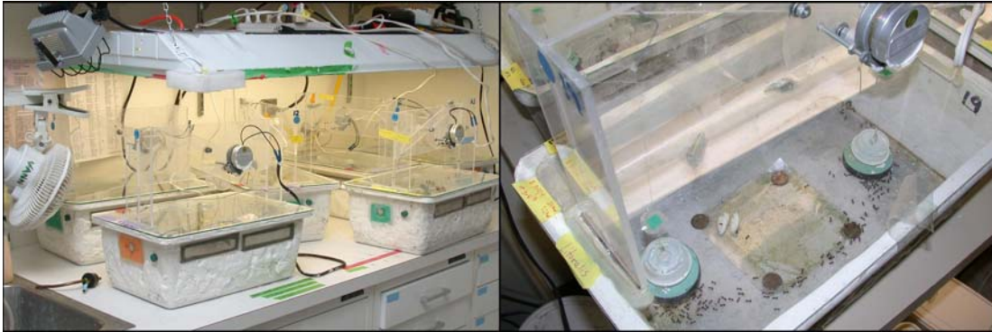
Figure 3. Attack boxes used in no-choice tests at the USDA quarantine facility in Gainesville, Florida. The electric motor on top of the box drives a cam that raises and lowers the green and black lids inside the box every 15 minutes so that ants trail back and forth while the flies attack. Photos: S. D. Porter.
