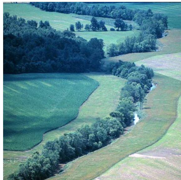
Figure IV-8: Riparian forest buffer and grass filter strip system
