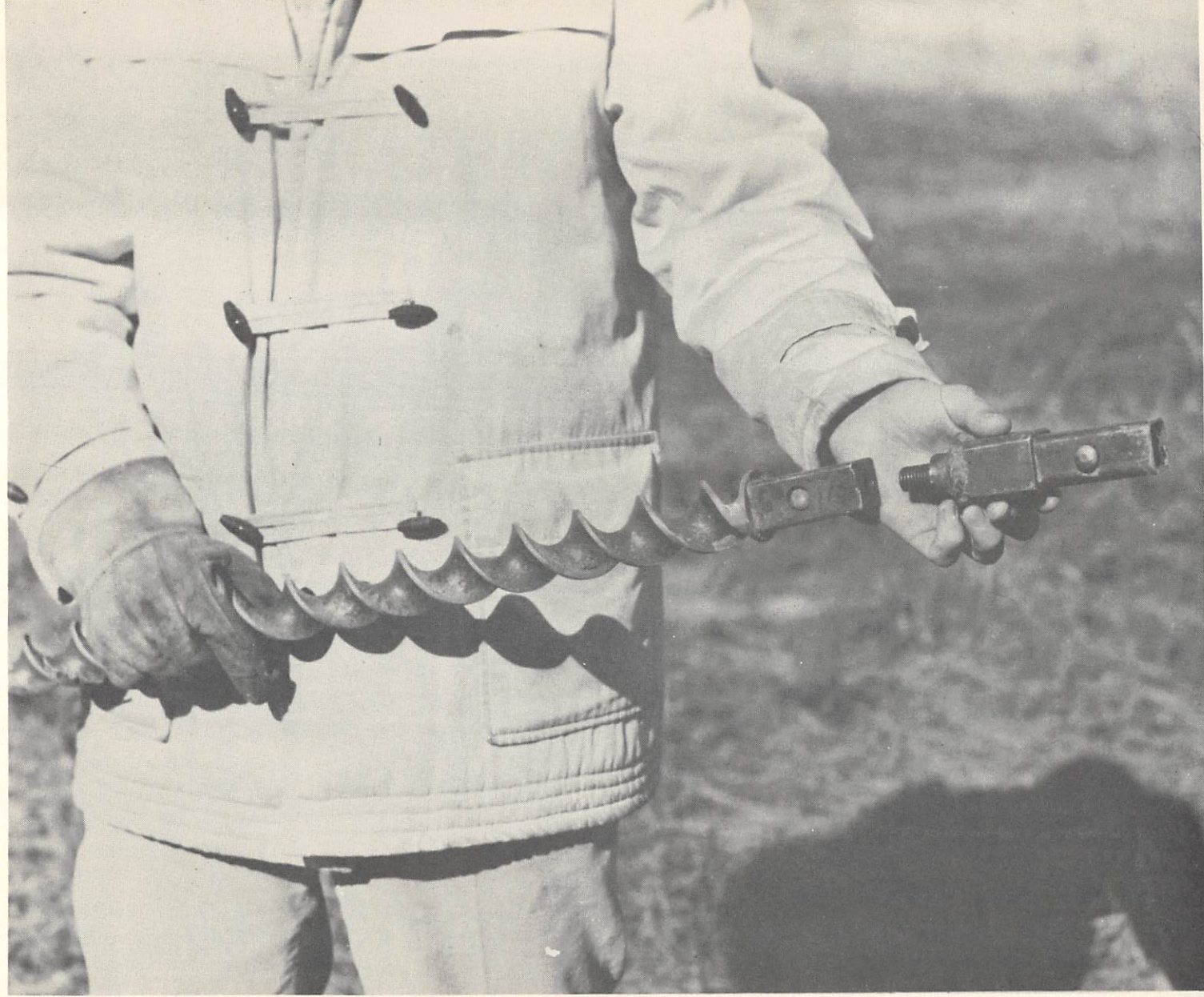
Fig. 3. Two-inch full-flight auger showing special adapter for attachment to power sampler.
