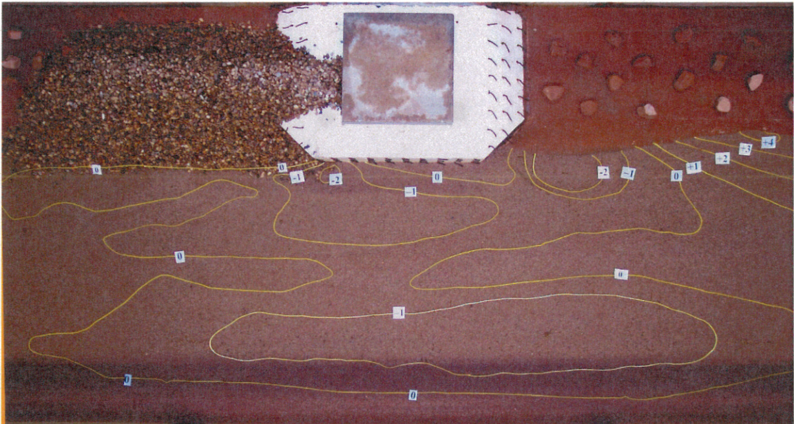
Fig. 6-7: Scour contour of Test 9. in Table 6-3 with gravel diameter 6.7~9.5 mm, 1.5L length, rock wall end slope H:V=30/13.2, side slope H:V=18/13.2, a small apron at the end . Wall base is even with abutment. y_m = 13.2 cm, y_f = 5.2 cm, Q = 0.0371 m 3 /s, t = 4800 min. Flow from left to right.
