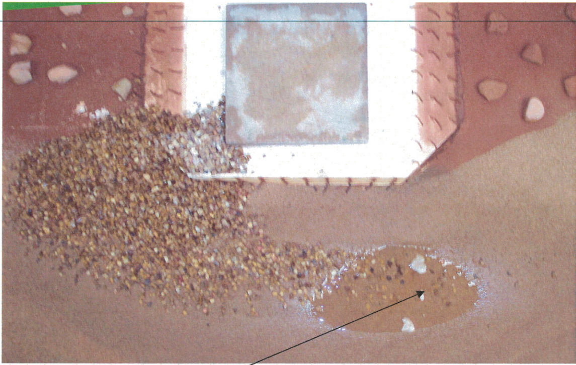
Fig. 7-1: Photograph of excessive scour around a poorly-positioned spur dike. (Flow from left to right.)
