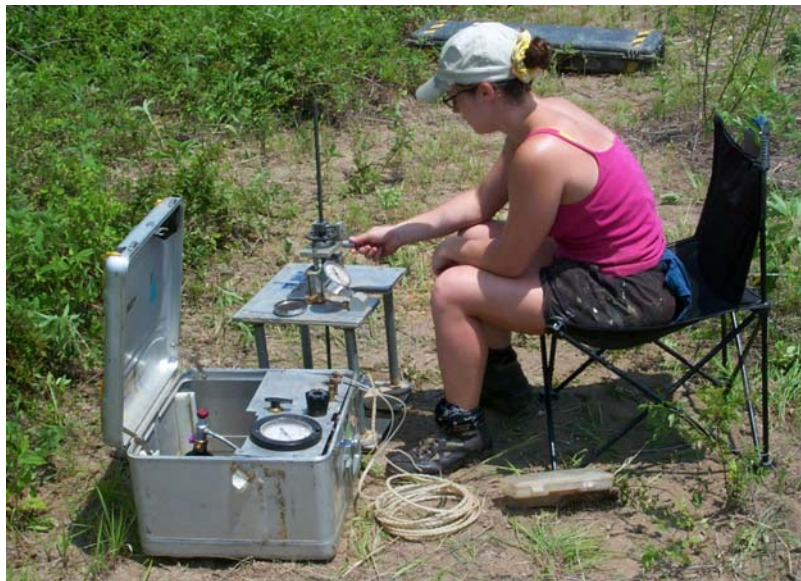
Figure 65 – Borehole shear-test device (BST) used to conduct tests of the shearing resistance of different layers of streambanks along James Creek.
