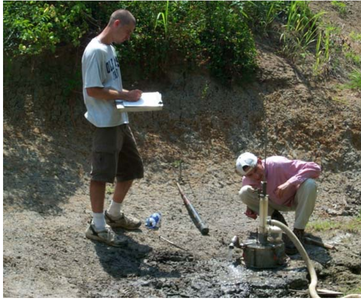
Figure 64 – Non-vertical jet-test device used to determine erodibility of bank toes.
