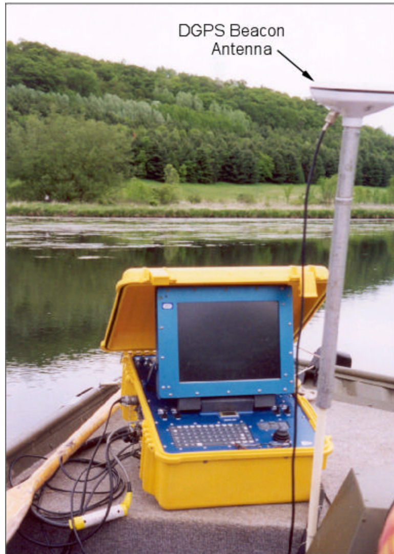
Figure 3-1. Photograph of acoustic profiler control module. All acoustic profiling and DGPS navigation electronics are contained in a compact, water-resistant control module.
