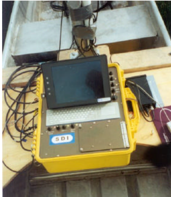
Figure 4-3. Photograph of acoustic profiling system (May 2001).
