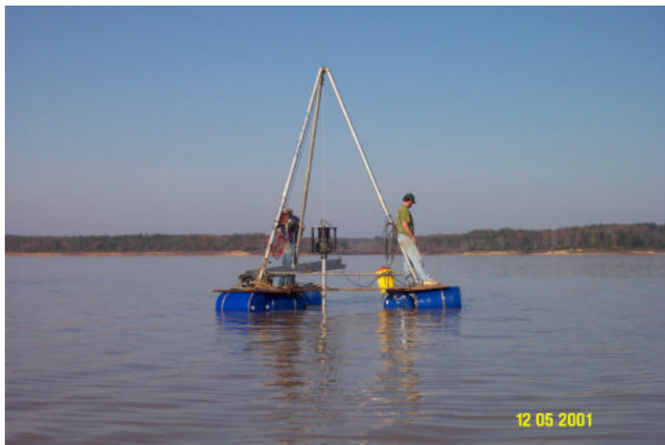
Figure 2-2. Picture of vibracorer taken on Grenada Lake.
