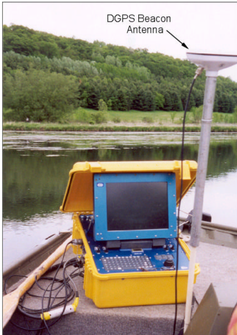
Figure 2-5. Photograph of acoustic profiler control module. All acoustic profiling and DGPS navigation electronics are contained in a compact, water-resistant control module.
