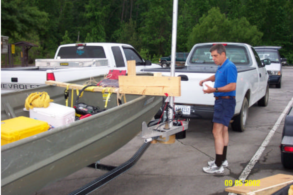
Figure 2-7. Picture of acoustic profiler transducer array mounted to the side of a Johnboat.
