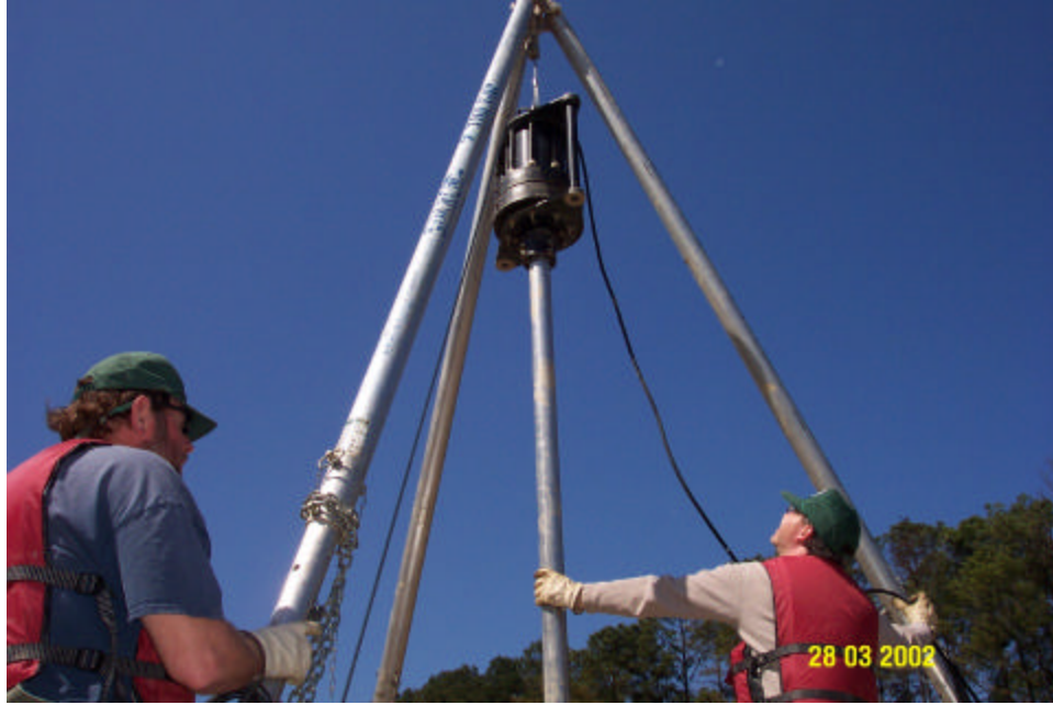
Figure 2-3. Picture of the vibracorer taken during operation on the Yalobusha River. Core pipe is fully extended.
