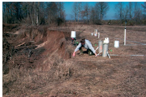
Figure 3. Determining bank retreat rate by measuring along established survey line on Little Topashaw Creek, Chickasaw County, MS
